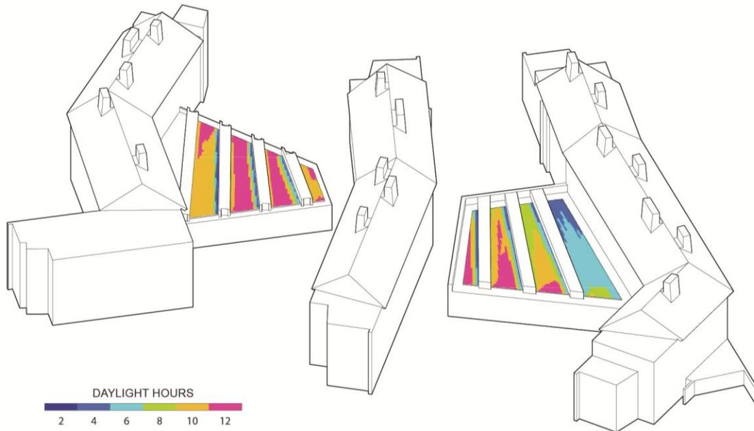
**Figure 5 Solar access analysis for House 1 (left) and House 2 (right).**
